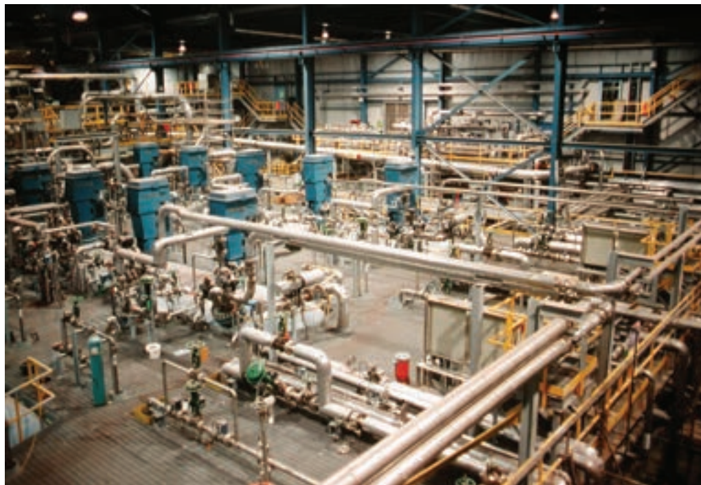
Figure 11: A view of the zinc pressure leach autoclaves and piping systems at Hudbay's Flin Flon plant (Gil Desrochers Collection HBMS EPSN 2036, Courtesy of the Flin Flon Heritage Project).
